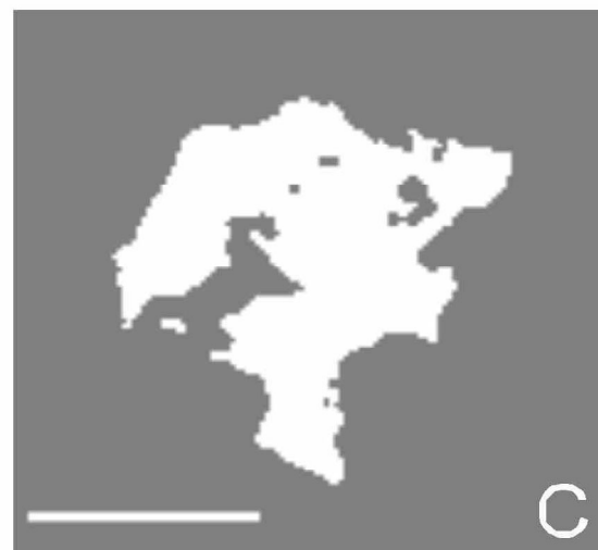
Figure 3: Derivation of contact boundaries from irm images. A typical IRM image of a THP-1 cell deposited on a polylysine-coated surface is displayed in Figure 3A (bar is 5 \mu m, contact time is about 2 minutes). The intensity profile along a line segment perpendicular to the cell edge (white line) is shown on B. Contact was determined by simple thresholding (C).
