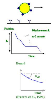
Figure 9. Studying individual ligand receptor bonds with a laminar flow chamber. The figure describes the use of a laminar flow chamber operated at very low shear rate.
