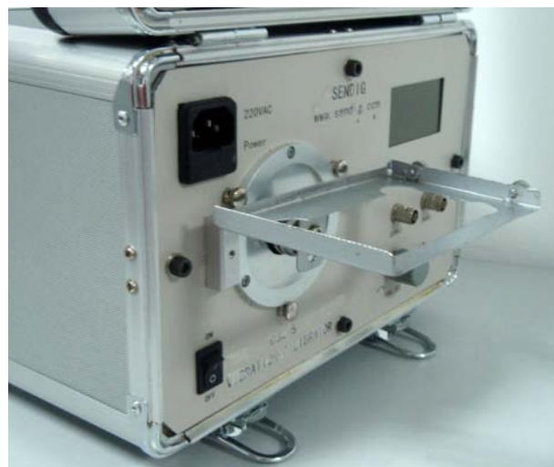
Fig. 2. View of GJX-5 vibration sensor and fixture.
