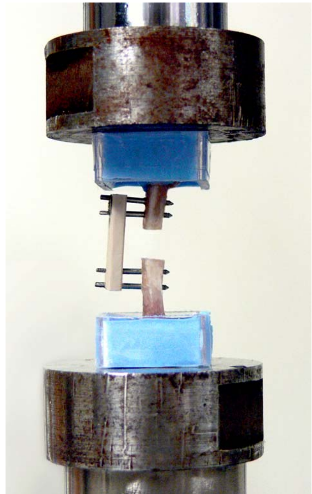
Fig. 4. Mechanical testing rig showing ExFixHigh assembled on a rat femur with a 5 mm defect.
