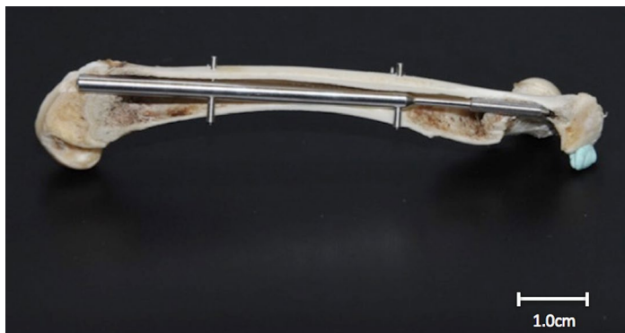
Fig. 1. RabbitNail in situ . The implant system contained a retrograde intramedullary nail that consisted of a distal shaft and a proximal threaded part with one proximal and two distal locking options ( \text{Ø} 1.00 mm). The nail shaft was connected to the proximal threaded part by a flexible shaft to adapt to the curvature of the femur. The function of the proximal threaded part was to engage the nail into the cancellous bony area of the trochanteric region of the proximal femur.
