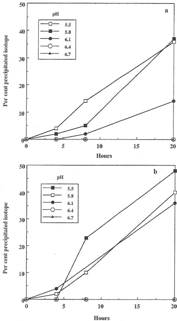
**Figure 3.** Precipitated [ $^{14}\text{C}$ ] oxalate during the first 20 hours following addition of CaP seed to Solution A without (a) and with (b) dialyzed urine at pH 5.5, 5.8, 6.1, 6.4 and 6.7.
